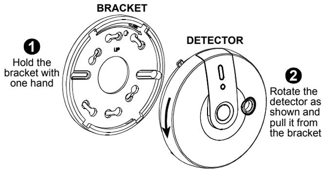
Figure 2. Separating the Detector from Its Bracket
