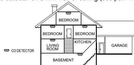
Figure 5. CO Detectors locations in a Multi-Floor Residence
